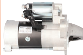
FORD RANGER 3.0 TDC1 4X WEAT 2007 - 2011 12V 10T 2.2KW
