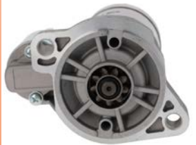
NISSAN HARDBODY 2.0i KA20DE 2003 - 2008 12V 9T 1.2KW
